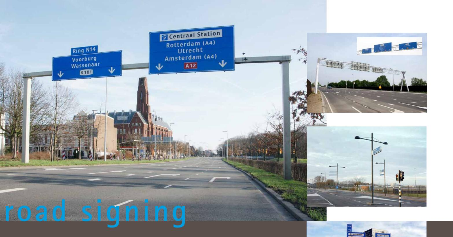
You want to install road signs alongside or above the road? PMF provides the design and the manufacture of the supporting constructions for static and dynamic road sign panels. We have a wide and deep assortment of poles and portals for your usage. The construction calculation shows the pole dimensions and the interplay of forces at ground level. The required foundation for the mast can be provided from this information.
